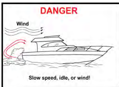
Figure 4.7. While underway or drifting slow speed can cause co buildup, add a tailwind and this can intensify the effect.
