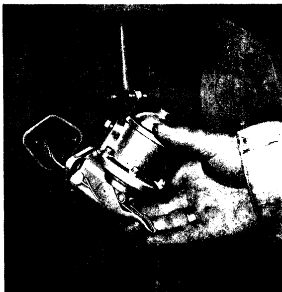
Fig. M.4. Removing Fuel Lift Pump.
