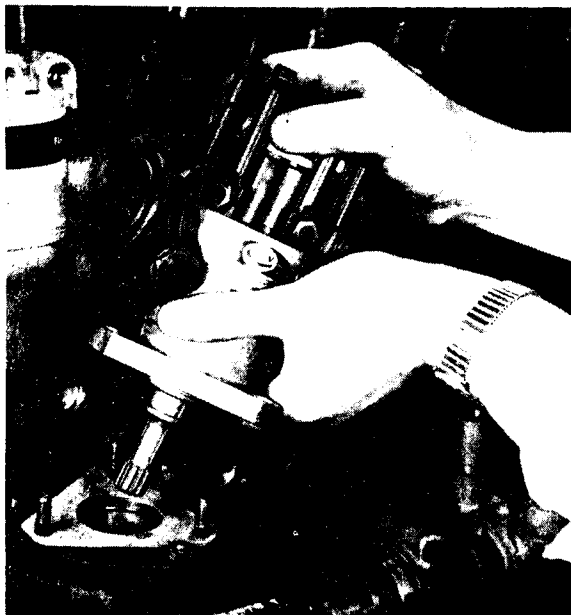
Fig. M.7. Removing Fuel Pump.
