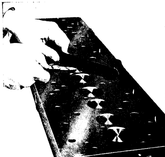
Fig. E.5. Checking Valve Depth.
