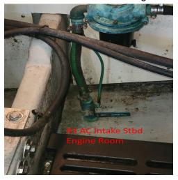
• Engine intake, thru hull (#5) and a strainer located aft of the engine in the engine room.
