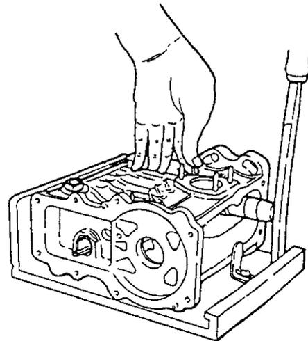
**NOTE:** 1. Be careful not to damage the oil seal with the threaded part of the camshaft.
