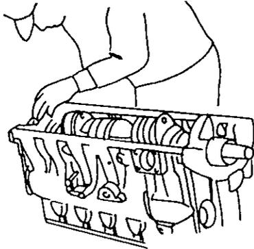
Fitting of thrust bearings
