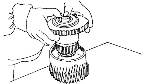
(2) Remove the pinion gears from the support shafts.
