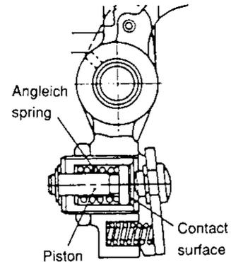
**Inspection of torque spring assembly.**
