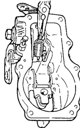
*Note: The governor assembly consists of the governor lever, tension lever, bushing, throttle spring and shifter, and is normally not disassembled. The spring pin is removed when you replace the shifter or throttle spring.*
