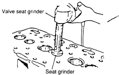
**NOTE :** Clean the valve and cylinder head with light oil or the equivalent after valve seat finishing is completed and make sure that there are no grindings remaining.
