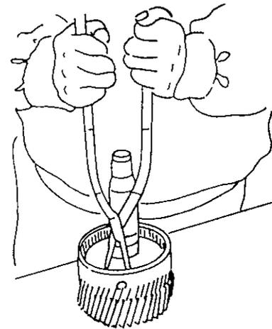
(4) Remove the circlip of the shaft by pressing the return spring several millimeters in a direction so that the spring goes away from the spring.
