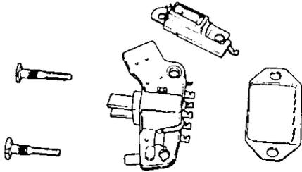
After repeating the above test, if any diode is found to be defective, replace the diode assembly. Since there is no terminal on the auxiliary diode, check the continuity between both ends of the diode.
