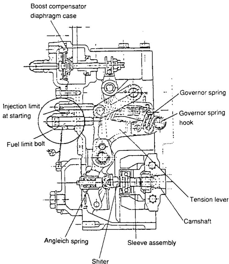
Before Adjusting the smoke cut spring assembly, adjust
