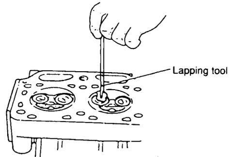
**NOTE :** Measure valve distortion after valve seat refinishing has been completed, and replace the valve and valve seat if it exceeds the tolerance.
