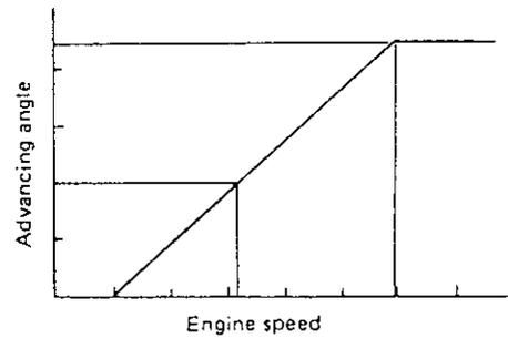
The advancing characteristics can be changed by changing the profile of the retainer guide groove of the weight and the spring constant and setting force of the spring.
