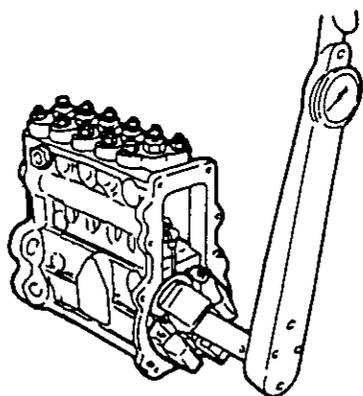
**NOTE:** Be careful as the taper fit comes apart after removing the nut ... the governor weight may fly out.
