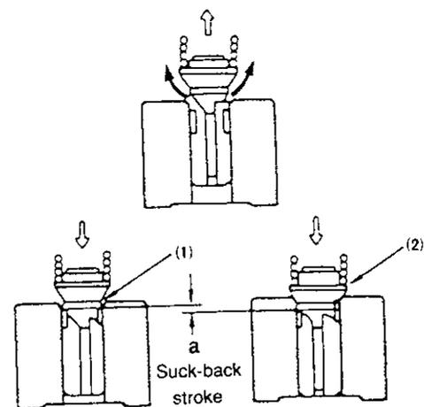
At the same time, the suck-back collar (1) blocks off the fuel injection pipe and the delivery chamber, and the valve continues descending until the seat (2) comes in contact with the barrel. The fuel oil pressure in the fuel
