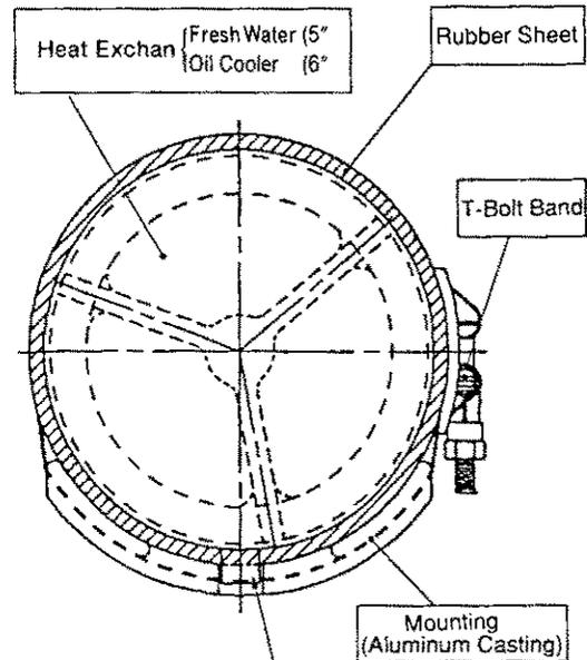
Check to see that the positioning pin is inserted in the hole.
