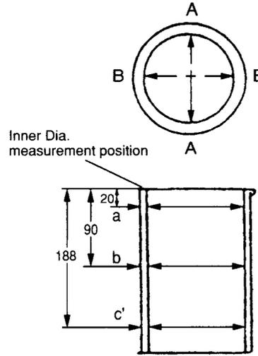
Note: Be sure to measure inner diameter of cylinder sleeve at points "a", "b", and "c" in directions "A" and "B".
