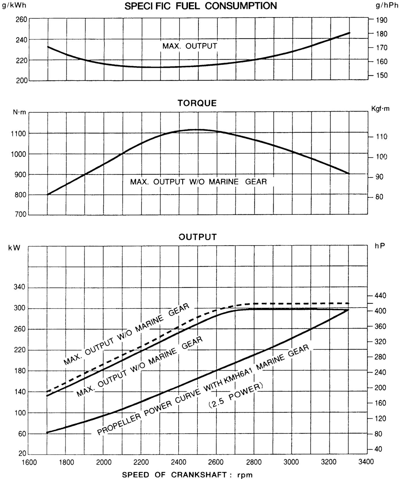
[6LY2A-STP (Fuel stop power : 324kW/3300rpm)]
