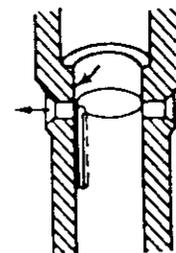
The delivery valve at the top of the plunger prevents fuel in the fuel injection pipe from flowing back to the plunger chamber and sucks up fuel from the nozzle valve to prevent after-drip.
