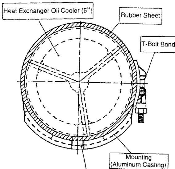
Check to see that the positioning pin is inserted in the hole.
