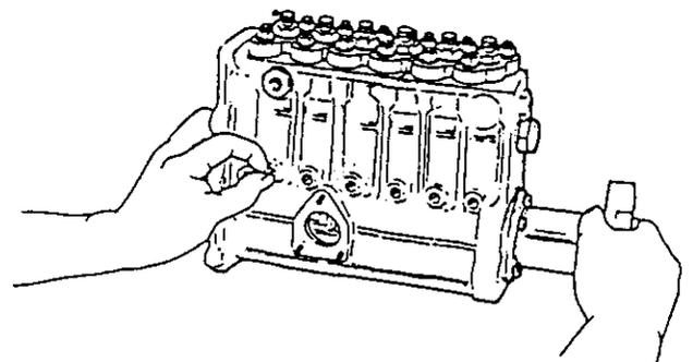
**NOTE:** If the camshaft does not turn, put double nuts or a coupling on the end of camshaft.
