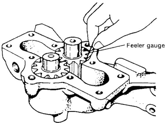
Measuring the oil pump gear-to pump cover clearance
