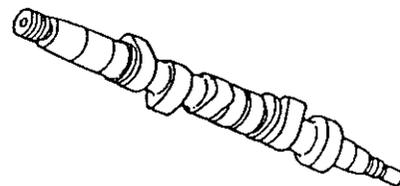
*NOTE: Replace fuel camshafts and bearings together.*
