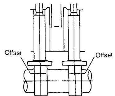
NOTE : When removing tappets, be sure to keep them separate for each cylinder and intake/exhaust valve.
