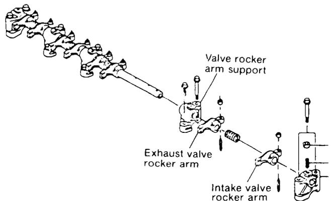
**(1) Rocker arm shaft and valve rocker arm bushing**
