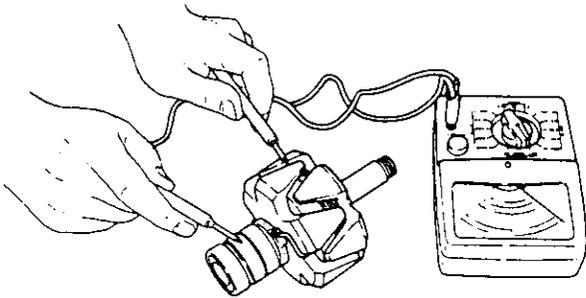
2) Stator coil insulation test
