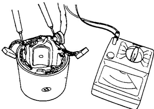
Field coil insulation test
