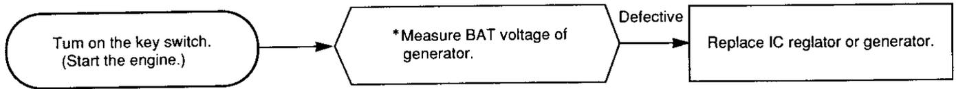
(3) Charge lamp failure
