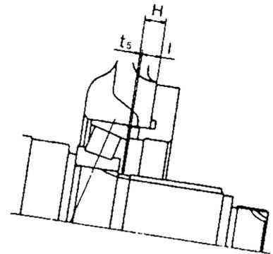
Adjust the clearance to the taper roller bearings.
