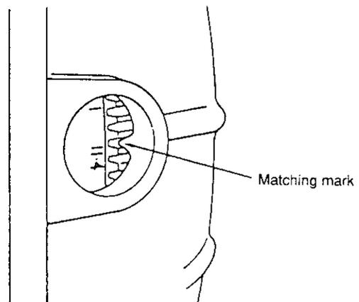
The matching mark is made at the hole of the flywheel housing.
