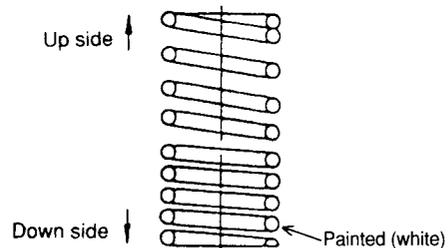
NOTE : The pitch of the valve spring is not even. The side with the smaller pitch (painted white) should face down (cylinder head) when assembled.
