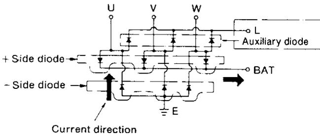
U.V.W.: terminal from the stator coil
