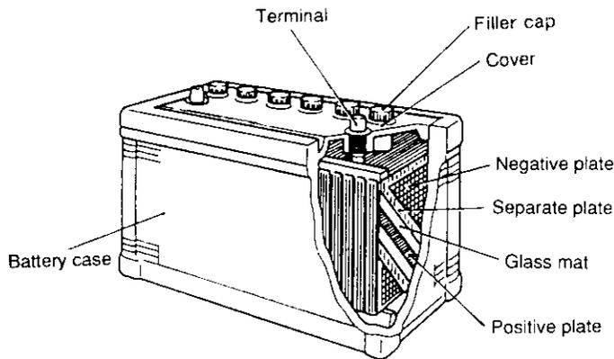
The battery utilizes chemical action to convert chemical energy to electrical energy. This engine uses a lead acid battery which stores a fixed amount of power that can be used when required. After use, the battery can be recharged and used again.
