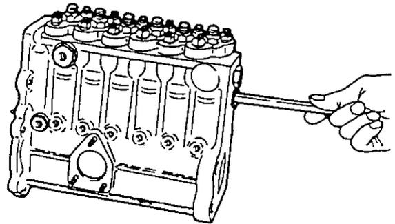
*NOTE: Be careful not to lose the spring and seats attached to the control rack.*
