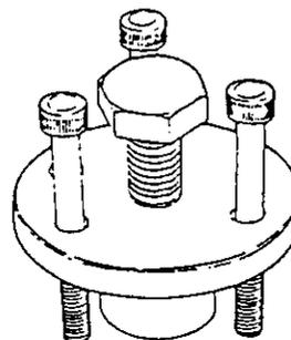
**NOTE:** The governor weight assembly is made up of the governor weight, support and pin. Do not disassemble.
