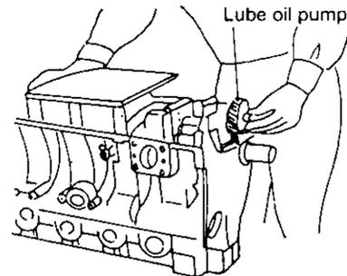
Fitting of lube oil pump idle gear
