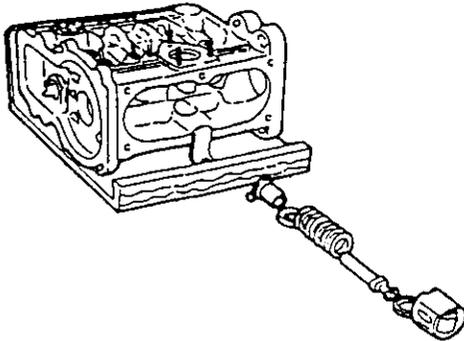
*NOTE: All of the roller guides will fall out when the fuel pump is stood up. So, first remove the roller guide support pin and roller guide for one cylinder at a time.*
