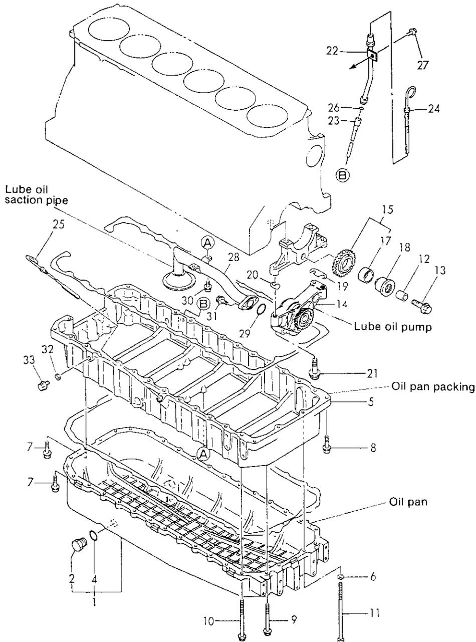
3-1.21 Remove the oil pan and the intermediate for the oil pan.
