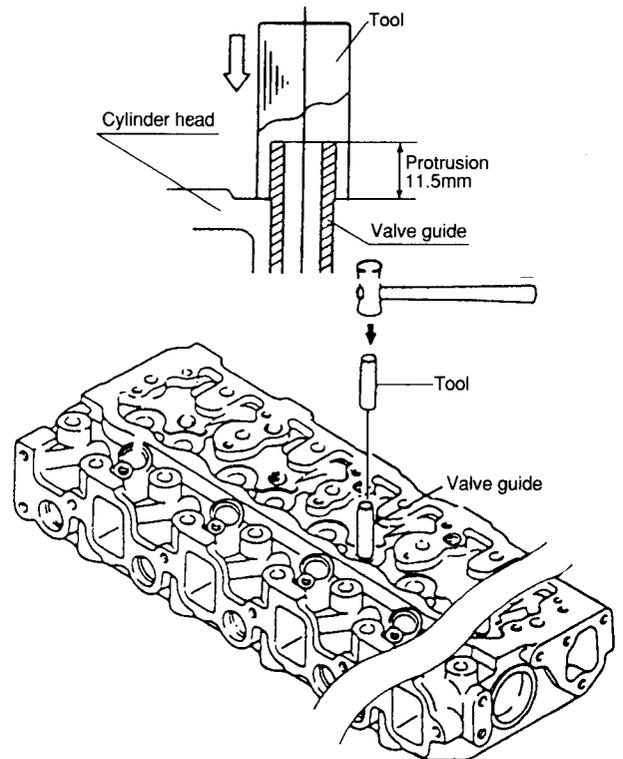
The intake valve guide and exhaust valve guide are of different shapes/dimensions.
