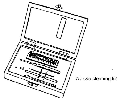
(3) Clean off the carbon on outside of the nozzle body with a brass brush
