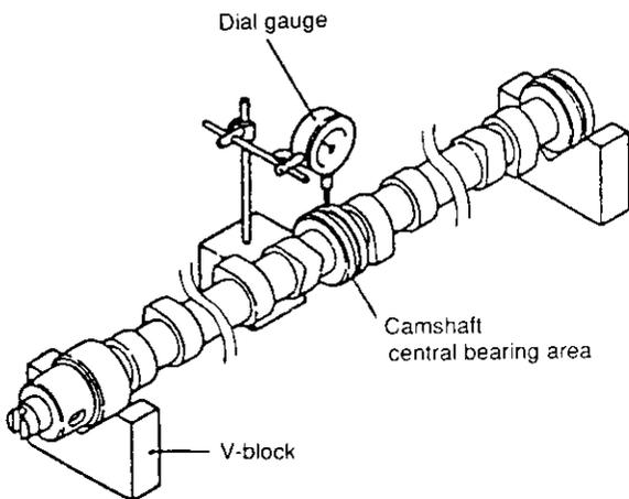
NOTE : The reading on the dial gauge is divided by two to obtain the extent of bending.
