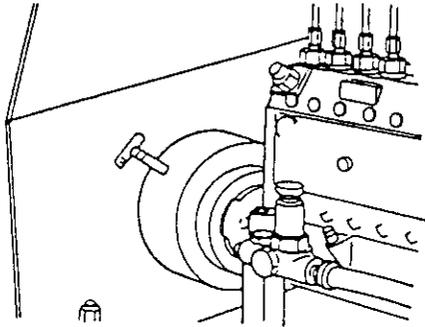
Fuel piping should be provided directly from the tank, not through the delivery pump of the tester.
