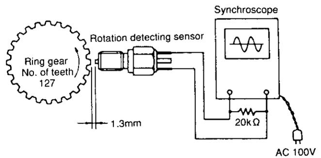
\*Check the output wave pattern and number of pulses when carrying out the output voltage measurement.
