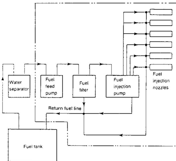
The Model YPES-6AL2 fuel injection pump is an in-line pump with a governor.
