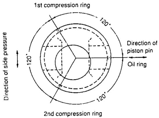
(5) The oil ring is provided with a coil expander. The coil expander joint should be opposite (staggered 180°) the oil ring gap.
