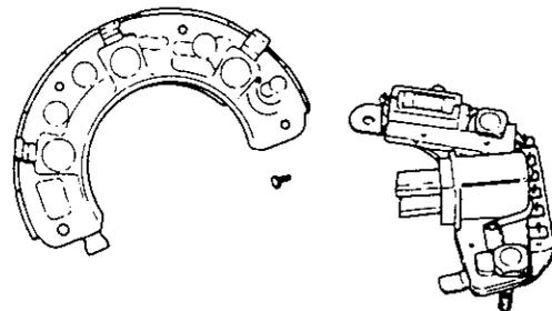
2) To replace the IC regulator, disconnect the soldered joint of the IC regulator and pull out the two bolts. Do not remove these two bolts except when replacing the IC regulator.
