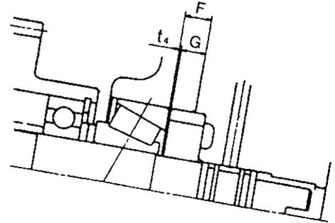
Adjust the clearance to the taper roller bearings.
