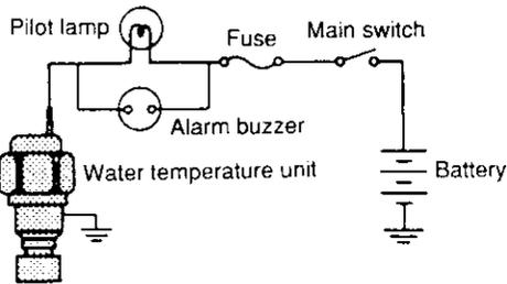
(Water temperature alarm circuit)
