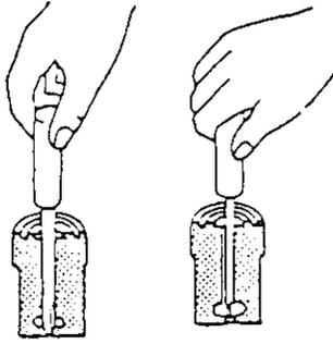
(6) Clean off the carbon on the tip of nozzle with a piece of wood.
