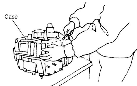
(11) Take out the support shaft assembly and output shaft assembly.
