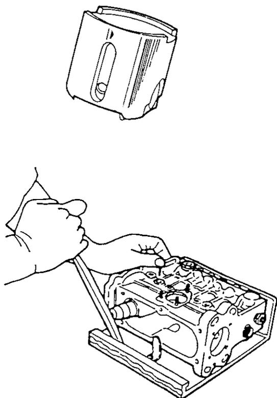
*NOTE: Check the movement of the rack. If the movement is heavy, the plunger spring may be out of place. Insert a screwdriver and bring it to the correct position.*
