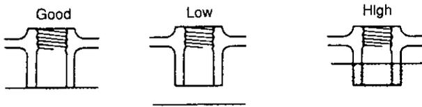
Check the electrolyte level every 7 to 10 days. The electrolyte must always be 10~20mm (0.3937~0.7874in.) over the top of the plates.
