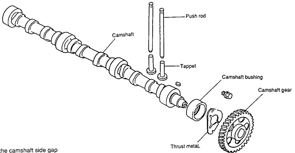
(1) Checking the camshaft side gap
